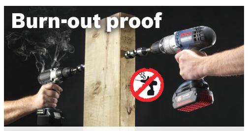
The 'smoking gun test'T: two combi's – one with ECP<sup>+</sup> and EMP<sup>++</sup> and one without. Stall the machine and keep pulling the trigger. Within seconds one tool starts to fry.
