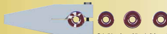
Rebuild surface of the shaft for a clamp connection
