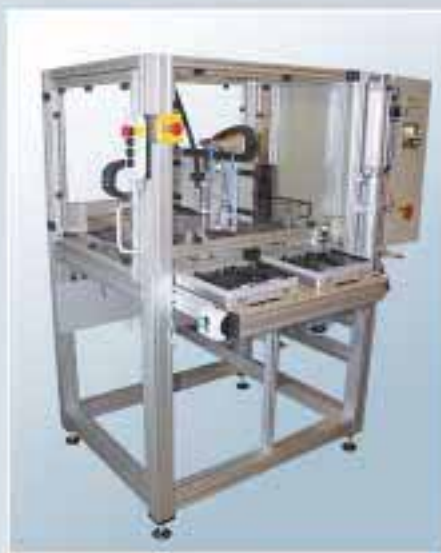
Automatic silicone gasketing dispensing with x-/y-robot
