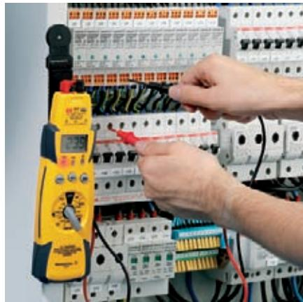
**Multimeter 2606****Digital clamp-on measuring device**
