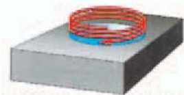
Plunge milling, circular
