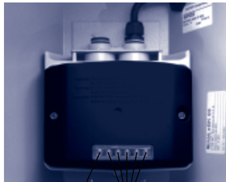
red LED green LEDs Monitoring display
