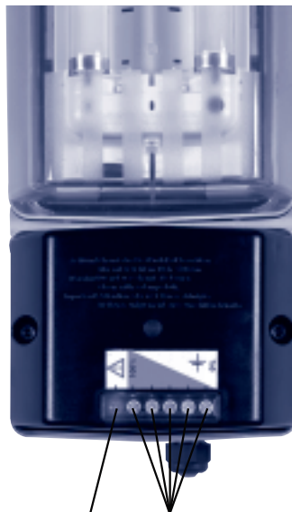
red LED green LEDs Monitoring Display
