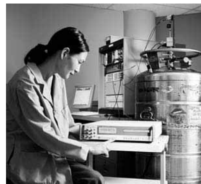
Josephson arrays in US and Germany. Fluke is only one of a handful of commercial organizations operating Josephson Array standards to represent the volt in their metrology operations. Fluke maintains two J-arrays, one at its corporate headquarters in Everett, Washington in the USA, and one in its standards laboratory in Kassel, Germany.
