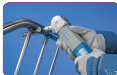
Head can be rotated through 180°
