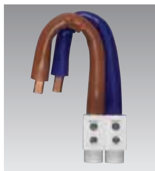
The incoming meter tail kit allows you to save time when installing 25mm 2 & 35mm 2 meter tails by simply connecting to the direct terminal block. This removes the need to bend incoming cables into the consumer unit.
