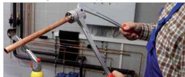
Quality protection against wear with the **TiN sealed** pin drive. Lifelong expanding precision
