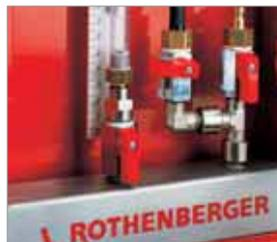
Adjustable scale to set the zero point measurement. Blue liquid for easier reading
