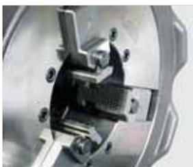
Automatic die heads with quick adjustment of thread size automatic thread length, finely adjustable thread depth without recentering
