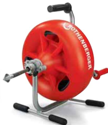
Set includes (No. 7.2003): Manual drain cleaner Type 3 S (No. 7.2003), spirals Ø 13 mm x 15 m (No. 7.2016), cross-blade cutter Ø 35 mm (No. 7.2176) and separating pin (No. 7.2100)
