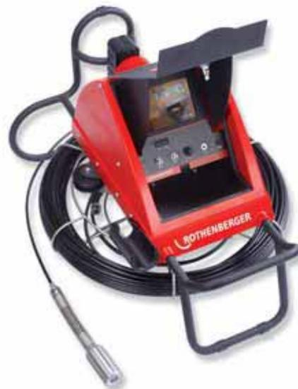
Largest pipe TV inspections camera with the new, self-levelling precision camera head that always shows an upright image. Registration of information and the use of drain software with an integrated damage catalogue (according to ATV), allows for high level documentation.
