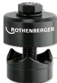
Metric tension screw with highest quality grade 12.9 (from Ø 15.2 mm)
