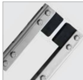
Simple replacement of electrodes and electrode holders
