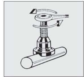
After extraction, set correct insertion depth (dependant on pipe Ø) with cam pincer
