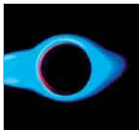
High flame temperature through cyclone swirl
