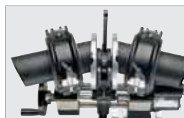
By adjusting the basic clamping element angles on both sides (15° each side) segmented bends can be produced
