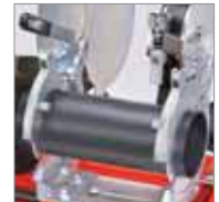
Basic clamping set for maximum diameter clamping
