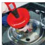
Electrical operation with cordless drill
