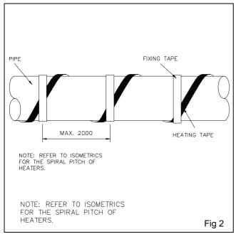
intervals than the 300mm recommended in most standards, eg. wrapping fixing tape in a continuous close spiral over the tracer is not good practice and may result in expansion failures near the mid-point of the circuit. It is sufficient to fix spirally applied heaters at 2m (6ft) intervals.
